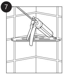
Apply silicon around each installation leg.
