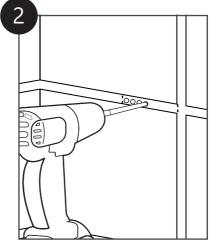
Pre-drill 1/8" pilot holes to 1/4" depth between the two marks
