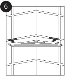
Insert install legs firmly into notches, right leg first.
