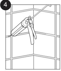
After removing spacers, clean out any remaining grit and apply silicon into each notch.
