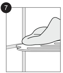
Wipe away excess silicon & clean residue with denatured alcohol.
