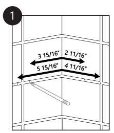
Mark out two, 2" wide notches onto the grout line.
