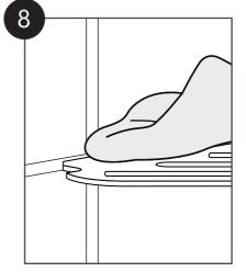
Wipe away excess silicon Clean silicon residue with denatured alcohol
