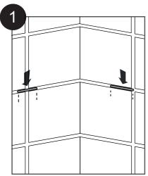
After completing tile installation, place 2" long spacers into install tab locations.
