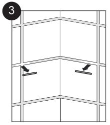
Carefully remove spacers after the grout is firm (or completely set).
