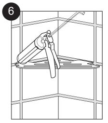
Apply a tiny bead of silicon around both install legs.
