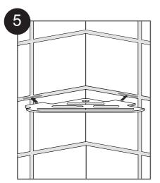
Insert install legs firmly into notches to at least 1/4" depth (right leg first).
