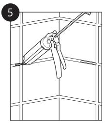
After cleaning thoroughly, apply a bead of silicon into each notch.
