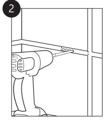
• Pre-drill 1/8" pilot holes to 1/4" depth between the two marks
