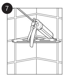
Apply silicon around each installation leg
