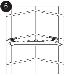
Insert install legs into notchesBe sure to insert the right leg first
